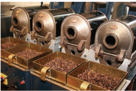
The cupping room micro roasters, fired by natural gas, roast the samples at between 300°F and 350°F for an average of about eight minutes.
